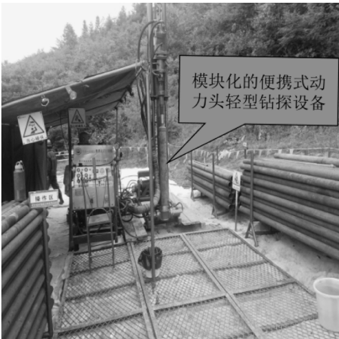
图 1 模块化轻型钻探设备 Fig. 1 Modular light drilling equipment
